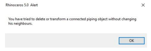
These modifications would have been alright if the piping element hadn't been connected (Try using the command "RP\_Disconnect" if needed), or if your selection contains all the connected piping elements.
