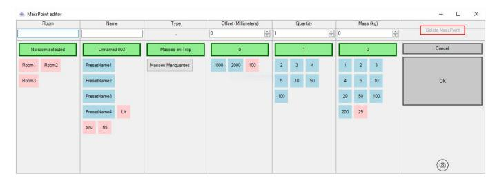
The light-red buttons are shortcuts to reuse the values existing in the model. The light-blue buttons
