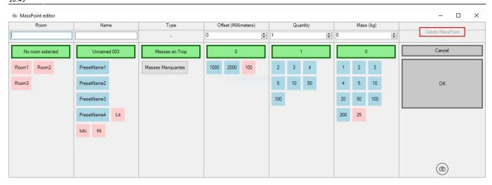
The light-red buttons are shortcuts to reuse the values existing in the model. The light-blue buttons are presets values defined in the LWS\_Options.
